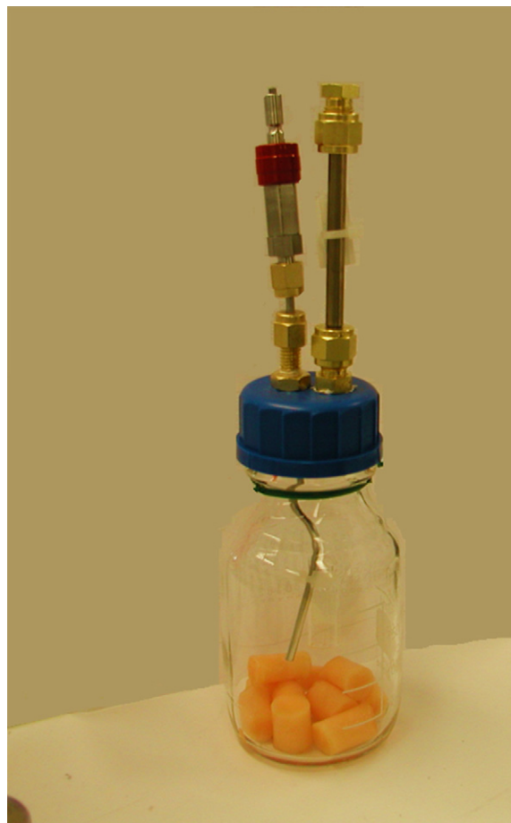
Fig. 1. Sampling bottle with specially transformed cap.
